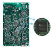
The double DSP based control system realized the digital control for all the power conversions of the UPS. Excellent performance is realized together with high reliability of the system.
